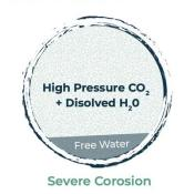
Historically, CO<sub>2</sub> pipelines have transported relatively dry and pure CO<sub>2</sub>. However, the expansion in different sources of CO<sub>2</sub> has the potential to lead to higher water content and more impurities introduced into pipelines. In addition, carbon dioxide mixed with water can form carbonic acid which is extremely corrosive to the internal surface of the pipe.
